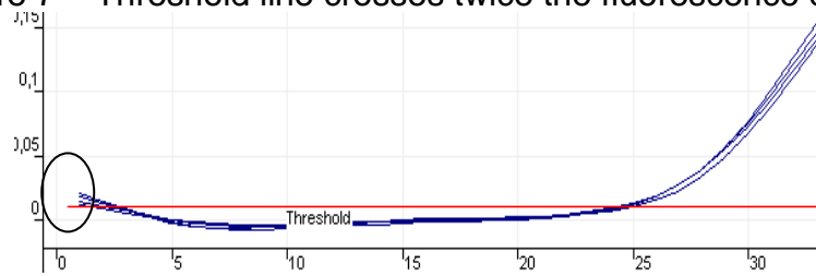
Figure 8 – Incorrect processing the curves with “bend” (from figure 2)
